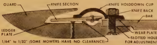
Figure 52. Relative position of a guard and its parts to the cutter bar.
